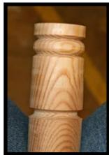
The skew is the best tool for cleaning endgrain and as Bill showed it is used long point down and then the handle is raised until the cut reaches the centre. The skew is the best tool to get into tight corners, e.g. when there is a need to cut right up to the revolving centre.
