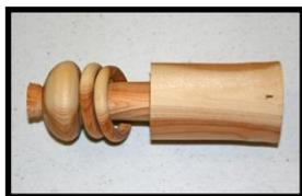
The final item Bill made was to demonstrate loose rings. He put a piece of Yew on the lathe, roughed it to a cylinder then made three incisions with a parting tool. With a skew he rounded over the tops of the "rings" and then with a tool he had ground to have a narrow hooked shape he undercut to release the two rings. The spindle was then narrowed down using a parting/beading tool. This project was not completed as can be seen from the picture.
